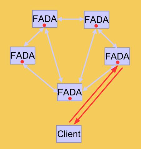
The service proxy is retrieved directly by the client, based on the Service locator delivered by the FADA node.
