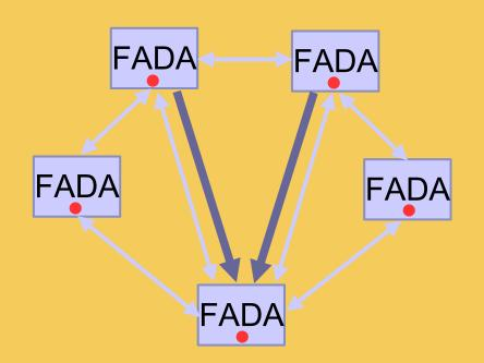
The latter neighbors notify their results to the first FADA node. As they weren't previously connected to the first FADA node, they connect inmediately.
