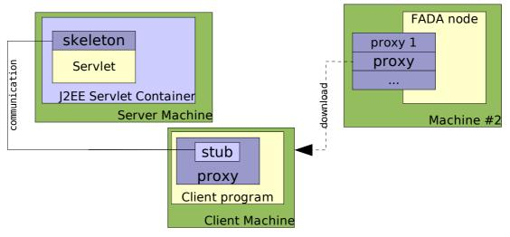
Registering a new proxy that contains the stub class
